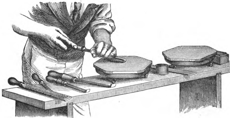
FIG. 8. Method of holding Scraping Tool.
